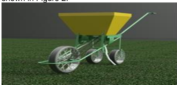
Figure 2. Isometric view of newly developed fertilizer applicator
